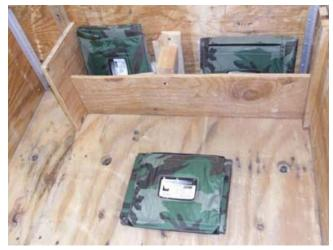
Three Global Solar P3 units were mounted in the cargo shaker unit, configured to each of the three required axes. The P3 units were subjected to fifteen minutes of loose cargo vibration according to each axis in three different fifteen minute intervals. After completion of the three configurations the P3 units were inspected for any irregularities. No irregularities were detected. (Fig. 1)
