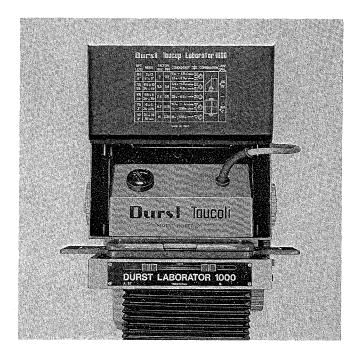
enlarger head in position with the knob (8) and only then withdraw the condensers. Push the TAUCOLI fully into the housing, then release the locking knob.
