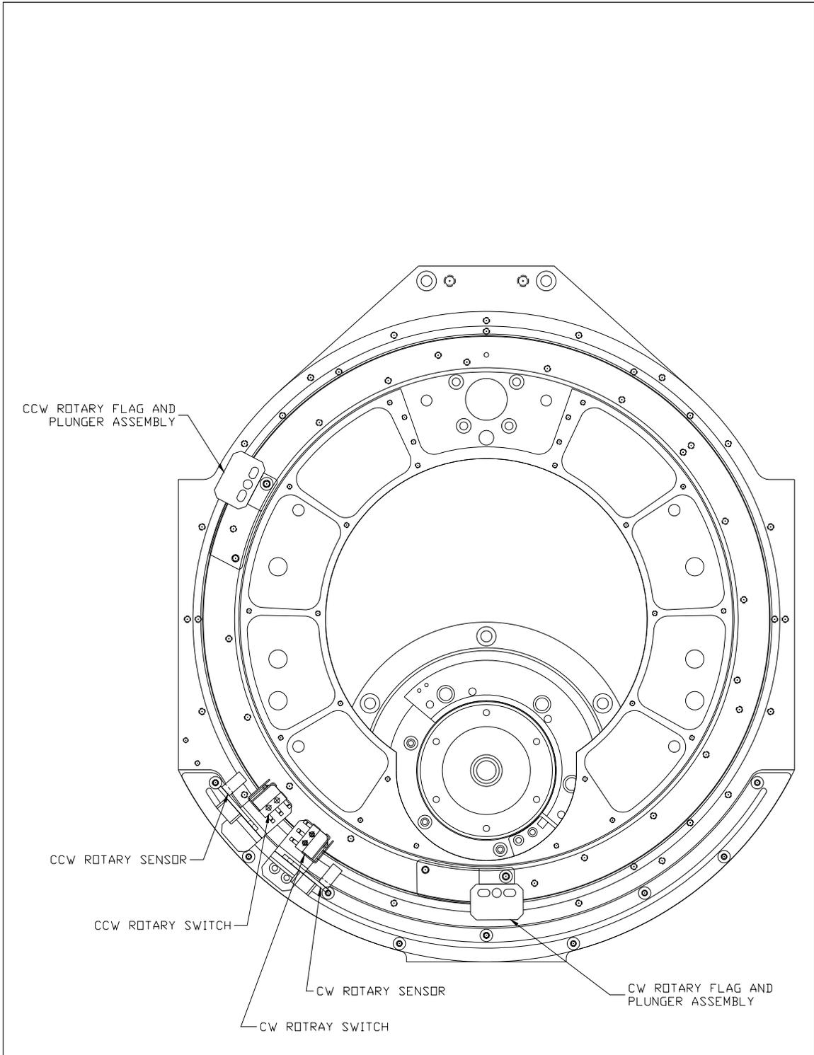
**Figure 8. Rotary Sensors And Switches**
