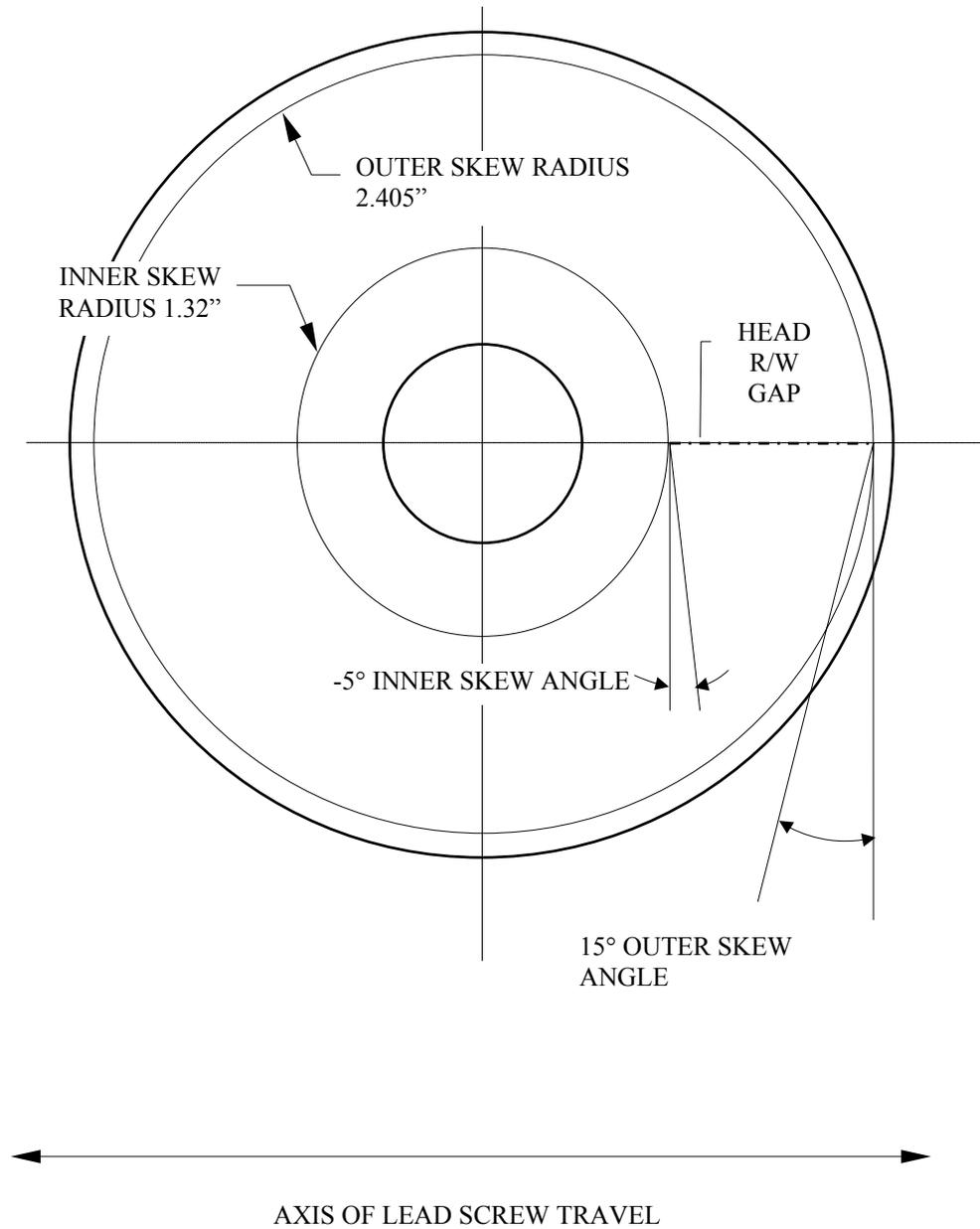
**Figure 2. S1701 Spinstand Skew Configuration Example**
