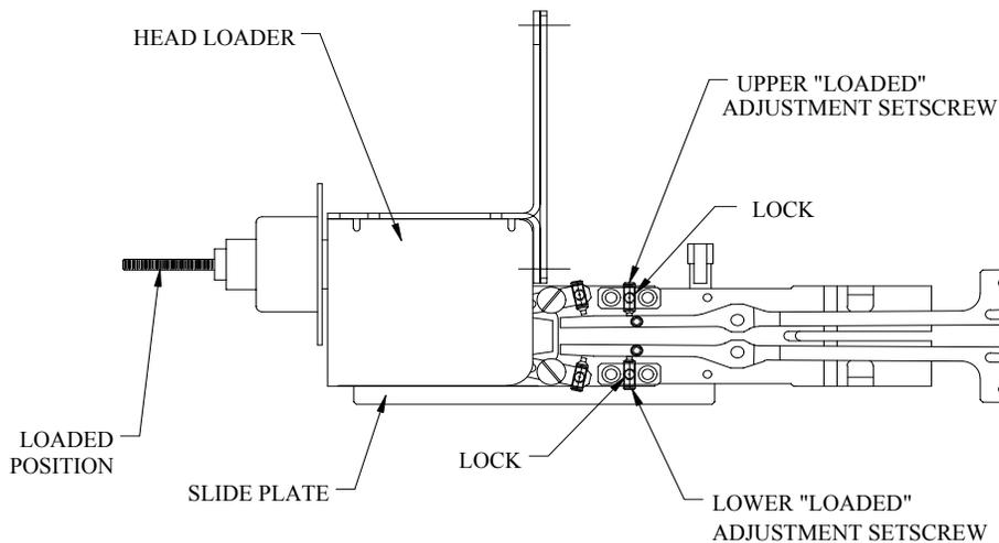
**Figure 15. Head Loading Mechanism “Loaded” Adjustment**
