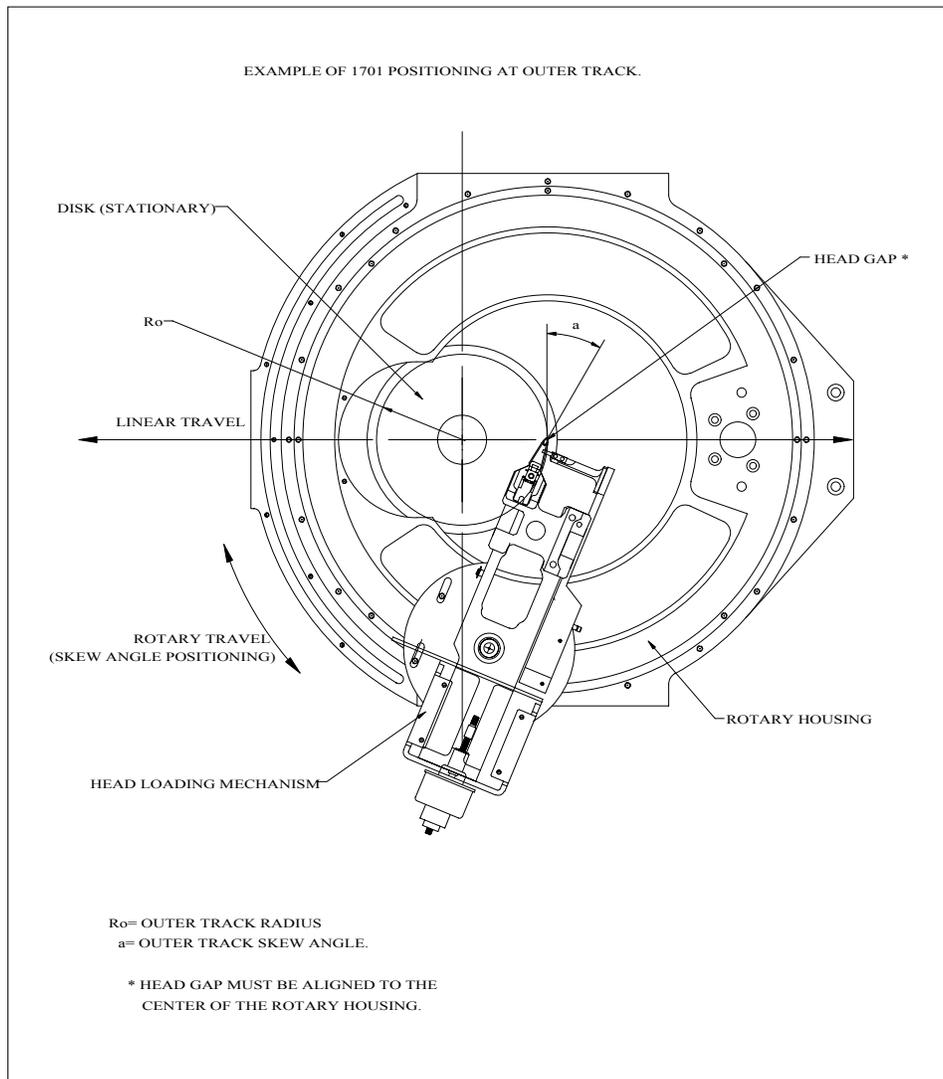
**Figure 4. S1701 Spinstand Positioning System At Outer Track**
