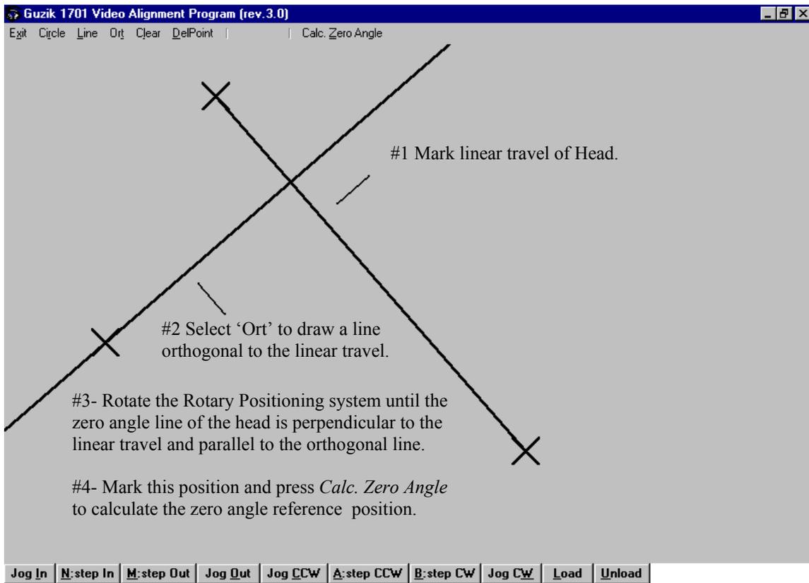
Figure 25. Locating The Zero Skew Angle Position
