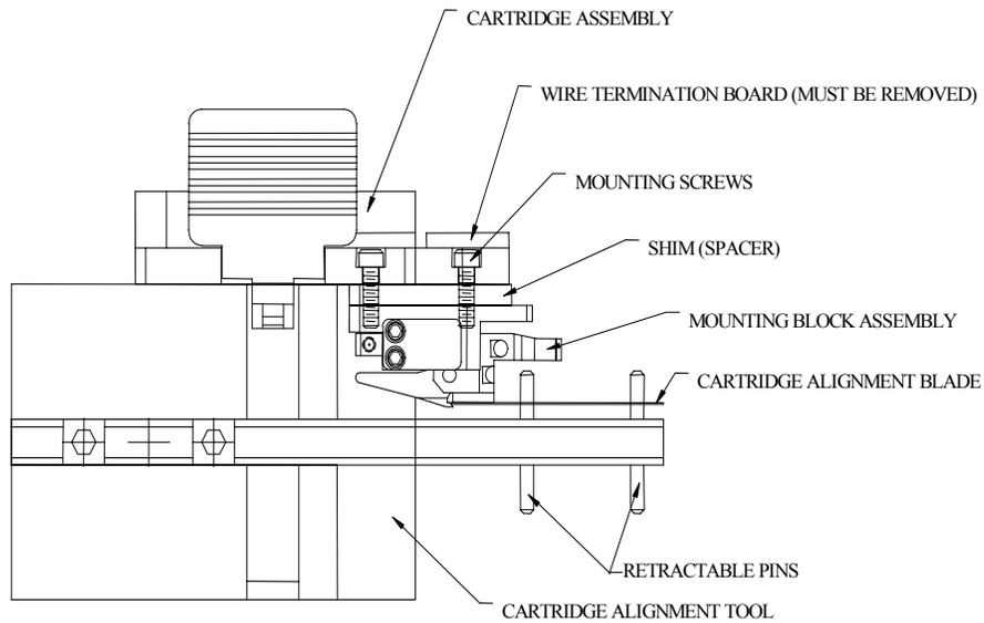
**Figure 13. Cartridge Alignment Tool**
