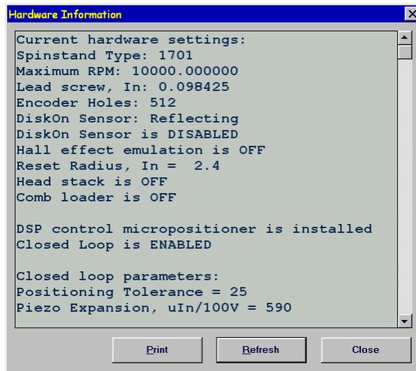
**Figure 29. Spinstand Hardware Information Window**
