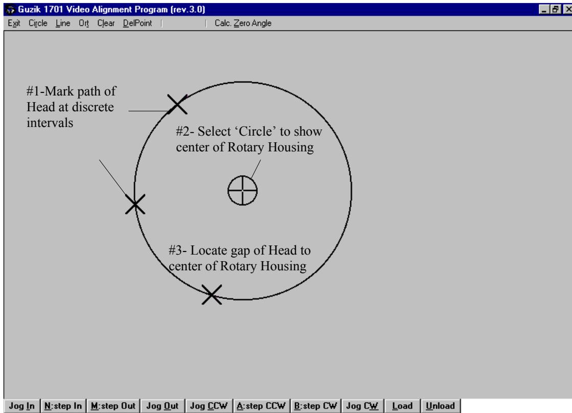
Figure 24. Aligning The Head Gap To The Center Of Rotation
