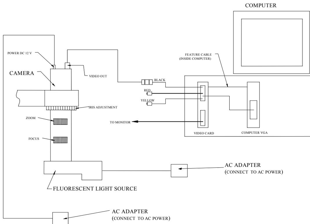
**Figure 18. Connecting The Optical Alignment System**
