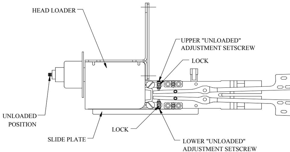
**Figure 14. Head Loading Mechanism “Unloaded” Adjustment**
