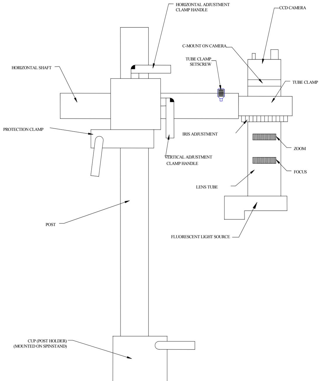
**Figure 19. Components Of The Optical Alignment Tool**
