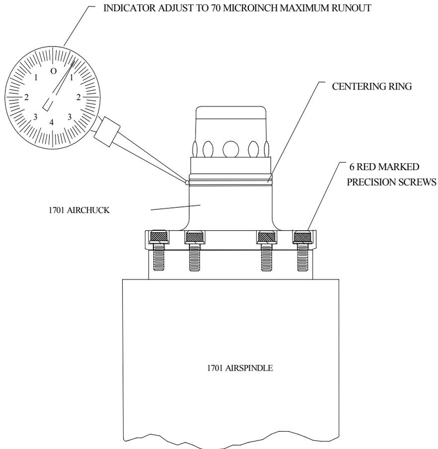
**Figure 10. Air Chuck Centering**
