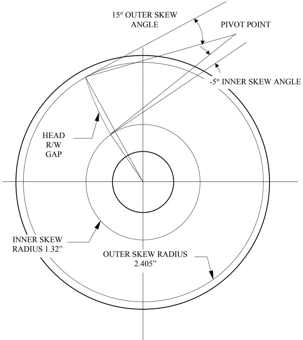
**Figure 1. Drive Skew Configuration**
