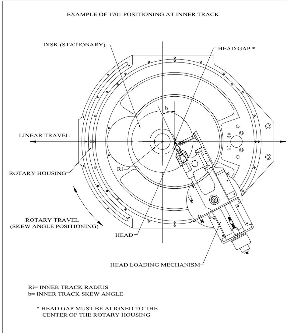
**Figure 3. S1701 Spinstand Positioning System At Inner Track**
